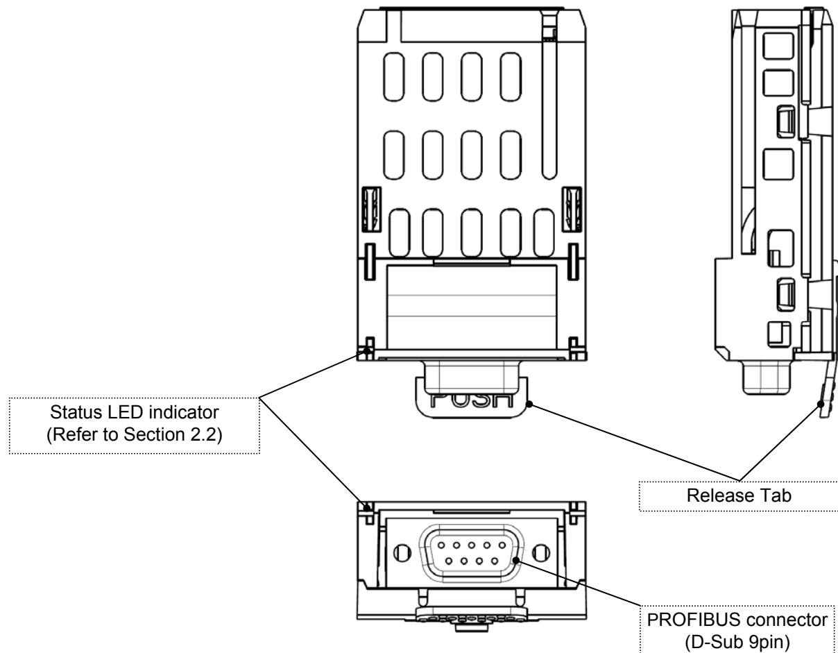
To align VF-MB1/S15 side-by-side horizontally, "Vertical" type PROFIBUS connector is necessary.
